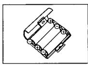
Insert the three R6 (AA, UM-3) size batteries observing the correct polarity.
